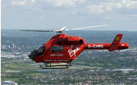
The London Air Ambulance (HEMS) operates a McDonnell Douglas Explorer helicopter based at The Royal London Hospital in Whitechapel, on a 24 hour basis. This aircraft is unlike many other helicopter types which fly over London because instead of a tail rotor, the MD Explorer is equipped with a no tail rotor system (NOTAR system). The NOTAR system provides the necessary anti-torque and steering control whilst eliminating the associated noise, thus making this aircraft much quieter to operate.
